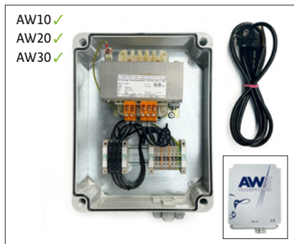
DRI-646 Transformer 230V/24VAC 500VA
